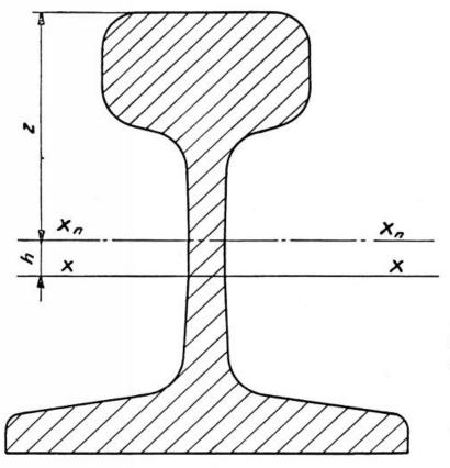
Set off the neutral axis  $x_n - x_n$ , adjust the rail to the line  $x_n - x_n$  as the new axis of moments, and again circumscribe the profile by means of No. 2 tracing point, taking readings on all the rollers. Thus:
