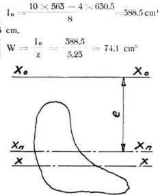
Large diagrams exceeding the range of the tracing point must be cut into smaller portions. If it is found impossible to follow the single portions with the tracing point after setting the rail of the Integrator to the axis of moments, an auxiliary axis parallel to the original axis of moments must be drawn for each portion.
