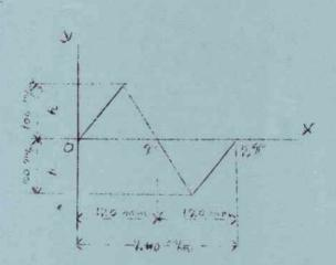
Take as example the isosceles triangle-wave line, drawn on 24 cm = 240 mm base with a height h of 10 cm = 100 mm (amplitude). Choosing two points of zero ordinate as limits of the wave portion to be analysed, the readings and the calculation of the corresponding harmonics are found as below. The figure was circumscribed 5 times for each harmonic and the average of the indications has been taken. The unit adopted is the millimetre; thus d = 20.
