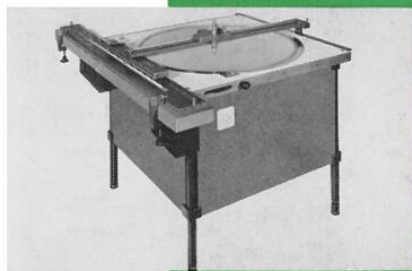
Coordinatograph with rotary table for industrial use
